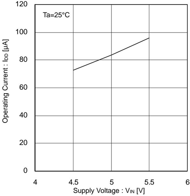
Figure 6. Operating Current vs Supply Voltage
