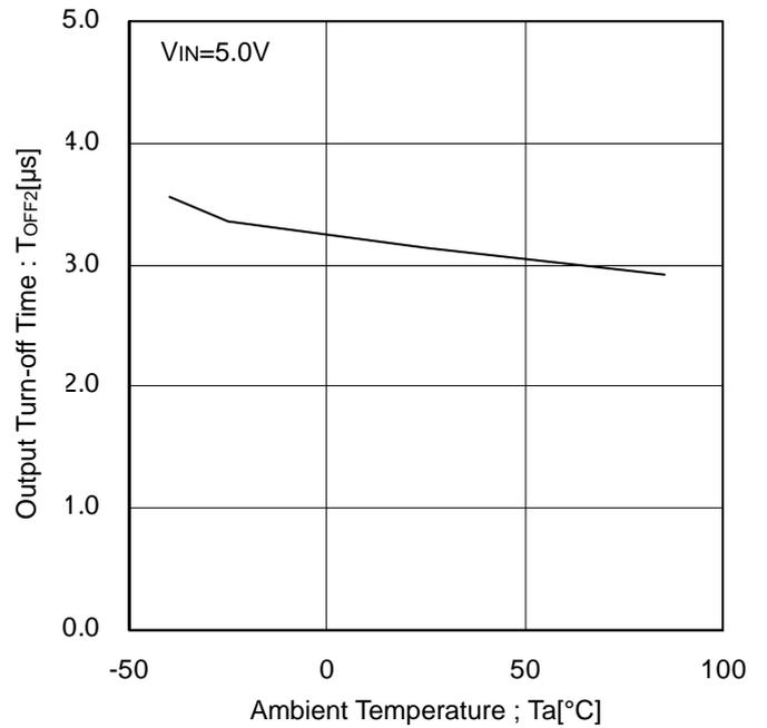
Figure 29. Output Turn-off Time vs Ambient Temperature
