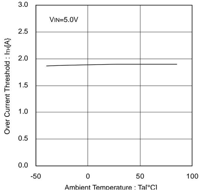
Figure 15. Over-Current Threshold vs Ambient Temperature
