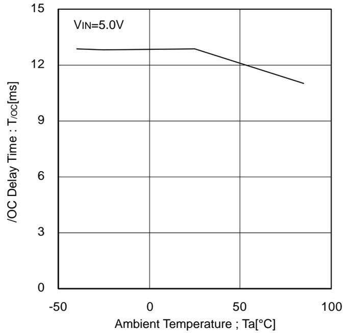
Figure 31. /OC Delay Time vs Ambient Temperature
