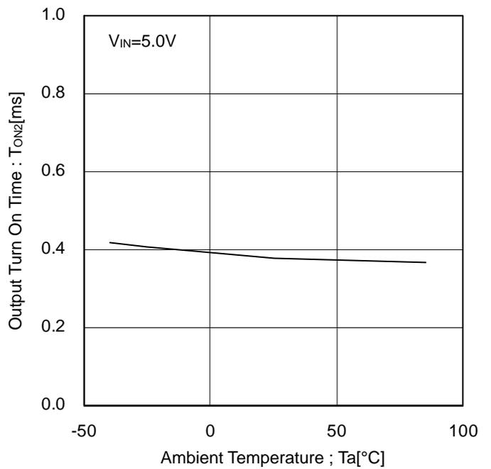
Figure 25. Output Turn-on Time vs Ambient Temperature
