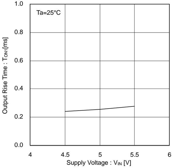
Figure 22. Output Rise Time vs Supply Voltage
