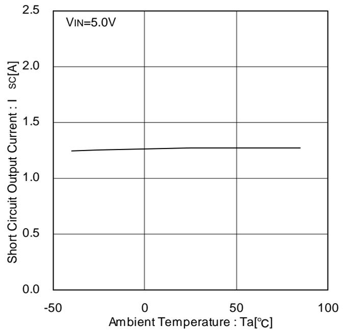
Figure 17 Short Circuit Output Current vs Ambient Temperature
