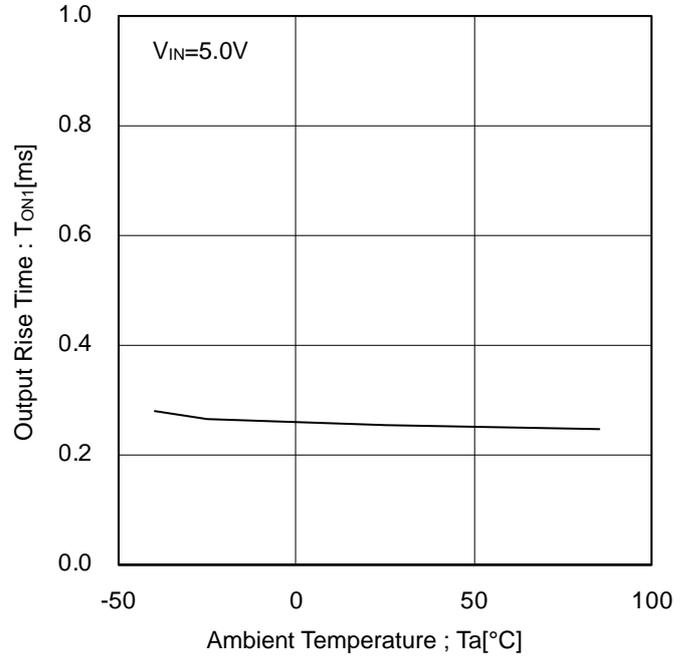
Figure 23. Output Rise Time vs Ambient Temperature
