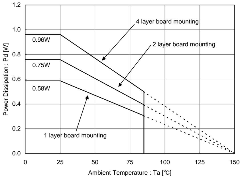
IC is mounted on 70mmx70mmx1.6mm glass-epoxy PCB. Derating is 4.7mW/°C above Ta=25°C.
