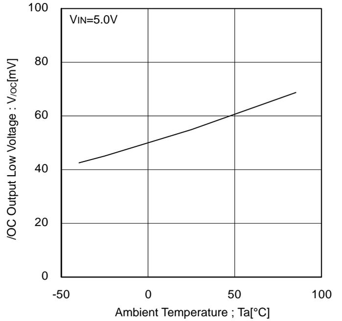
Figure 19. /OC Output Low Voltage vs Ambient Temperature
