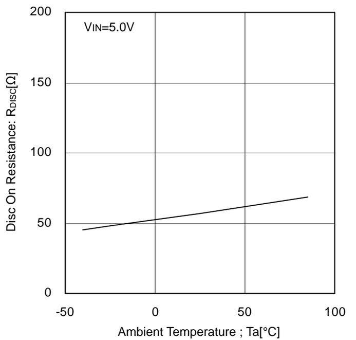
Figure 33. Discharge On Resistance vs Ambient Temperature
