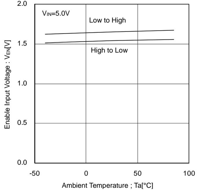
Figure 11. EN Input Voltage vs Ambient Temperature
