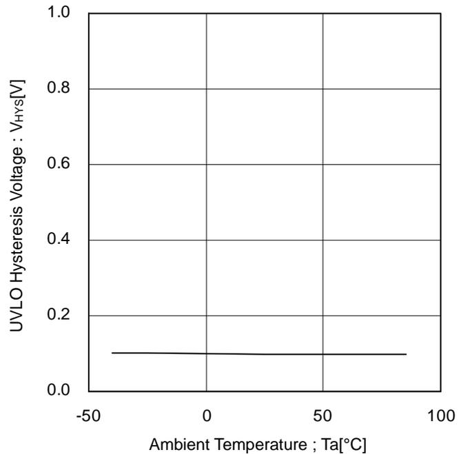
Figure 21. UVLO Hysteresis Voltage vs Ambient Temperature
