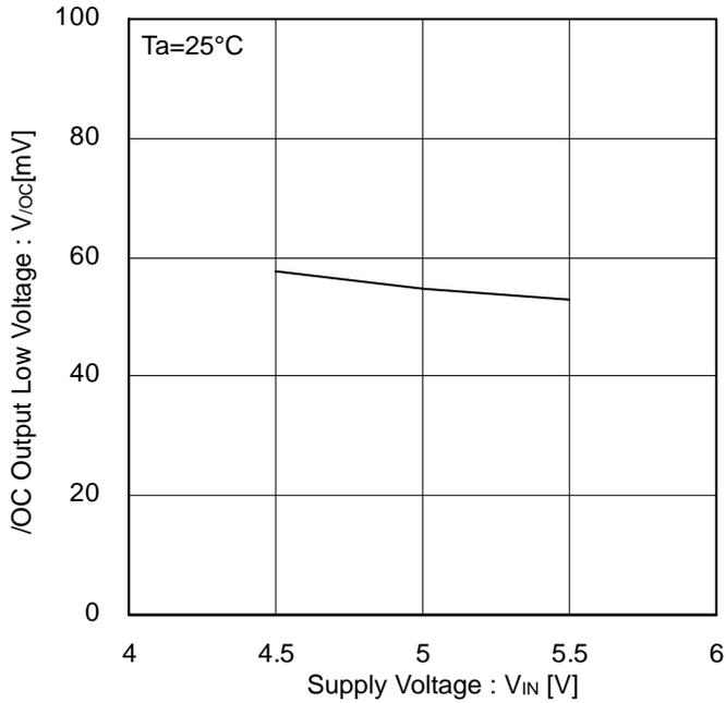
Figure 18. /OC Output Low Voltage vs Supply Voltage
