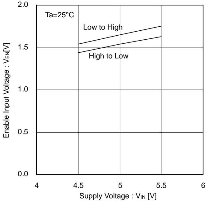
Figure 10. EN Input Voltage vs Supply Voltage
