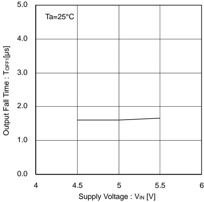
Figure 26. Output Fall Time vs Supply Voltage
